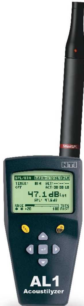
Acoustilyzer AL1 with MiniSPL Microphone
